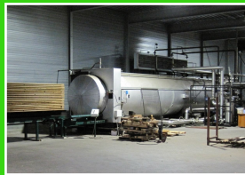
Thermal modification using pressurized steam in an industrial-scale autoclave at Firmolin BV (NL)
